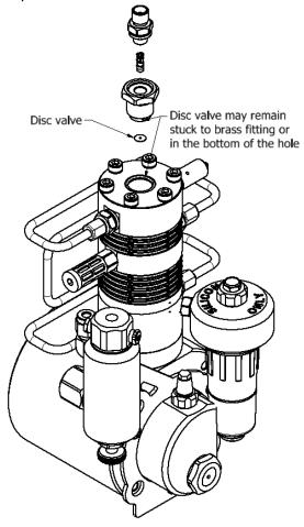
b. Ensure that that the disc valve is not bent whilst removing it.
