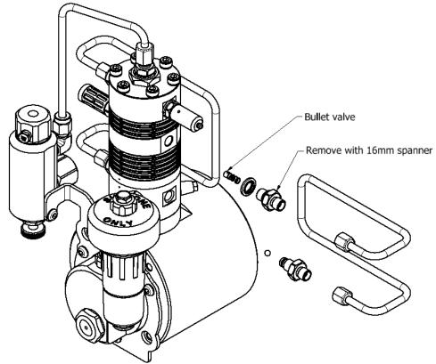
5. Remove pipe on left hand side of compressor head.
