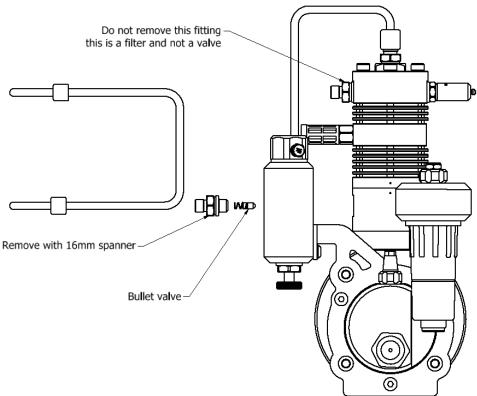
7. Remove middle left ball valve. It may be necessary to use a small object such as a craft knife to remove the ball from the compressor.
