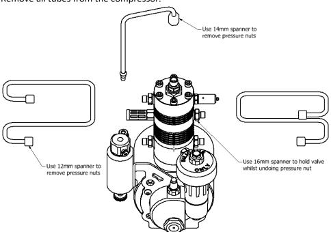
2. Remove 6 M5 bolts from compressor head.
